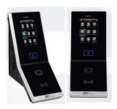
ProFAC is an access control terminal with RFID and face detection capability. With ZKTeco's latest ZKFACE version 7.0 high-speed face recognition algorithm and ZMM220 hardware platform (1.2GHZ clock rate), it has extremely high verification speed and low error rate. The ProFAC can hold up to 2000(1:N) facial templates, 4000 (1:1) facial templates, and 10,000 RFID cards. It is compatible with third party controllers and devices like electric door locks, alarms, door bells, and door sensors.
